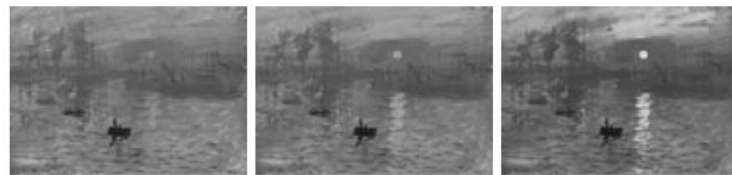
Figure 6: Changing the \alpha parameter: \alpha = 5, 10, 25 , respectively. Increasing alpha increases the contribution from chrominance differences but may cause dynamic range mapping problems ( \theta = 45^\circ ).
